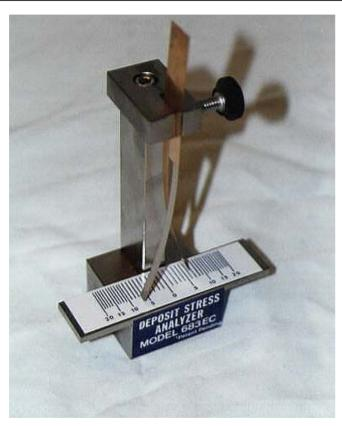
Monitor internal stress with convention coupon (dual beam made of alloy194)
