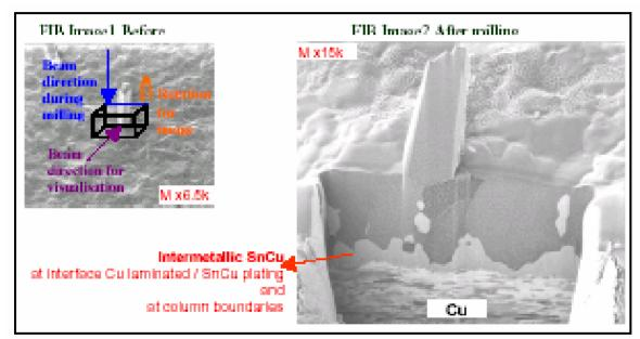
Images 1 and 2 are obtained by FIB—before and after milling respectively.
