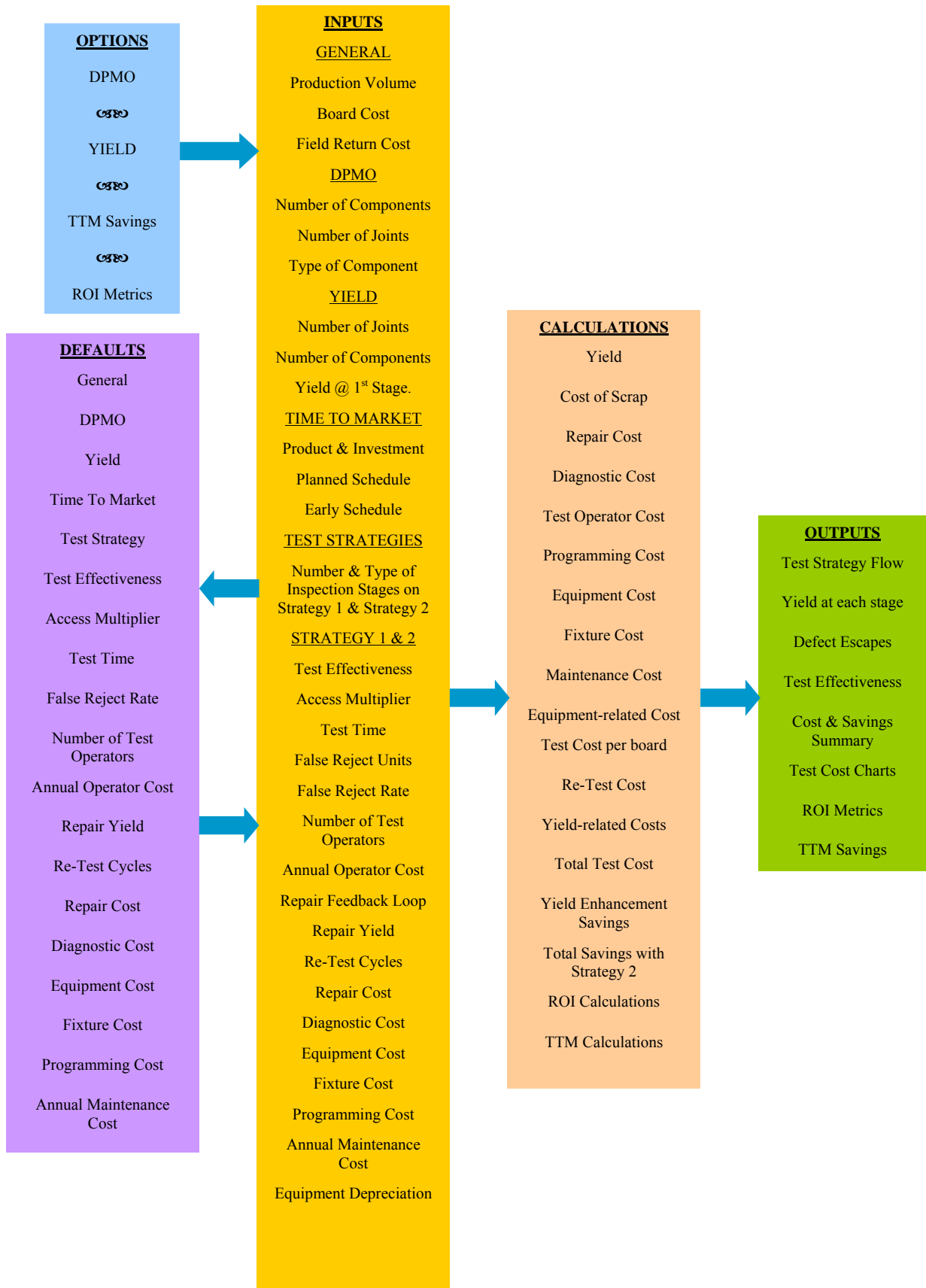
Figure 1 Four Major Sections of the Test Cost Model: Inputs, Defaults, Calculations & Outputs.
