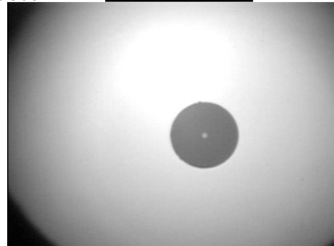
Clean Reference connector before the mating
