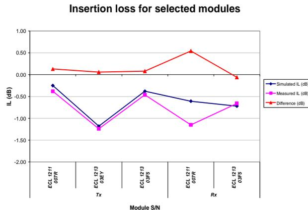
Figure 4: Comparison of Modeled and Measured IL
