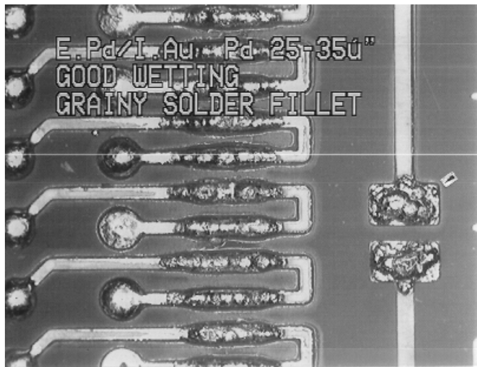
Figure 4 - Grainy Solder on Thick Palladium after Thermal Cycles
