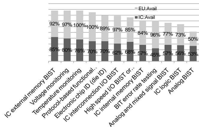
Figure 4 IC BIST tests available at the board level
