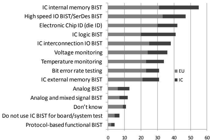
**Figure 10 Types of IC BIST run at the board/system.**
