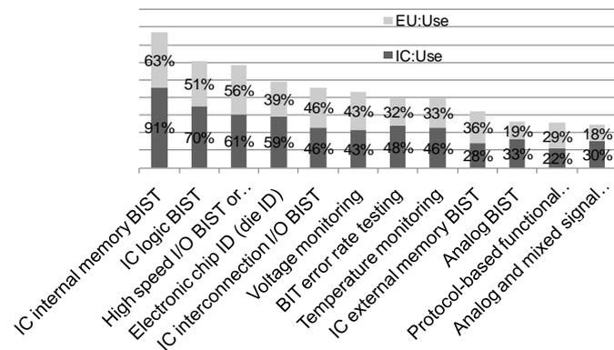
Figure 3 IC BIST availability at the component level
