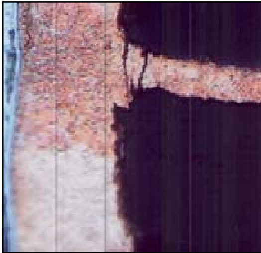
Crack in PWB (Laminate) Barrel
