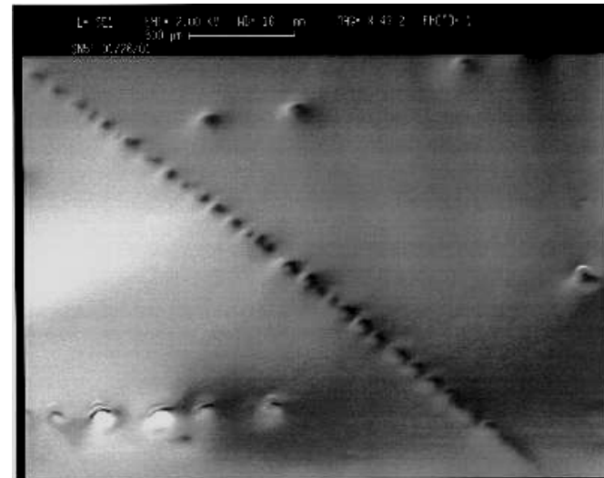
Whiskers growing “underneath” 2-mils of Polyurethane conformal coat. (Source: Mike Sampson, NASA)
