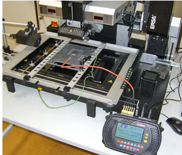
Figure 6: Typical setup of rework machine temperature measurement equipment placed in the rework machine
