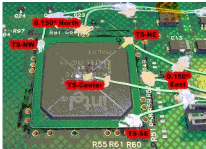
Figure 2: Topside thermocouple locations
