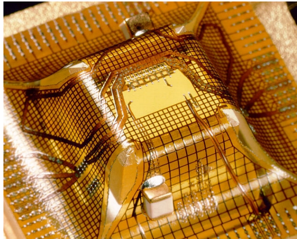
Fig. 3. An RF membrane probe core. This interfaces the chip under test to the probe card board. Probe tips around the rectangle in the center connect to a 50-ohm input line (lower right), a bypass capacitor (lower left), and a 2.5-ohm matching network and bias chokes (top).
