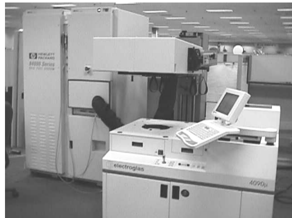
Fig. 1. An Agilent 84000 RFIC test system and Electroglas 4090 autoprobe. The test head is raised from its position of operation. Not illustrated is the operator’s workstation.
