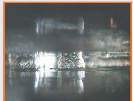
FIGURE 4: Differences in appearance between lead-free solder joints (left) and eutectic solder joints (right).
