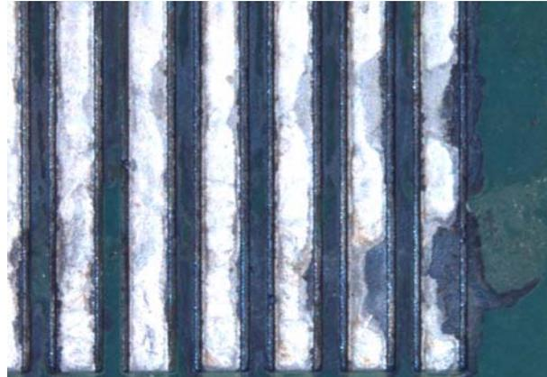
**Figure 12:** Pb-free HASL test board that was wave soldered with organic acid flux.
