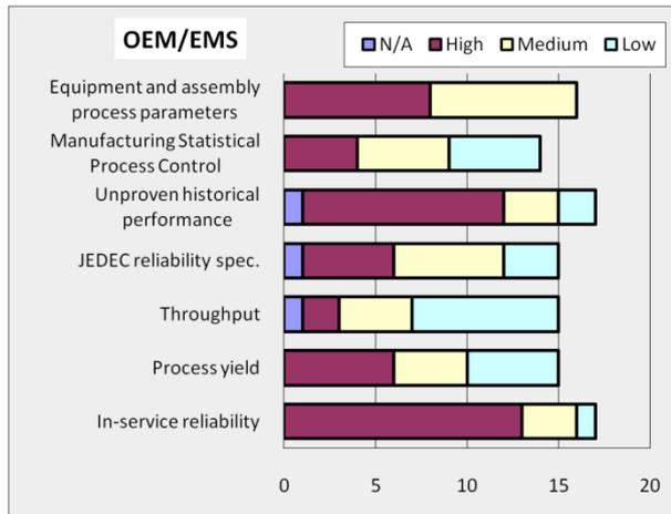
Fig. 4 Concerns with Cu Wire Bonding
