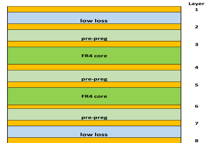
Multilayer PCB X-section with outer layer Microwave laminate
