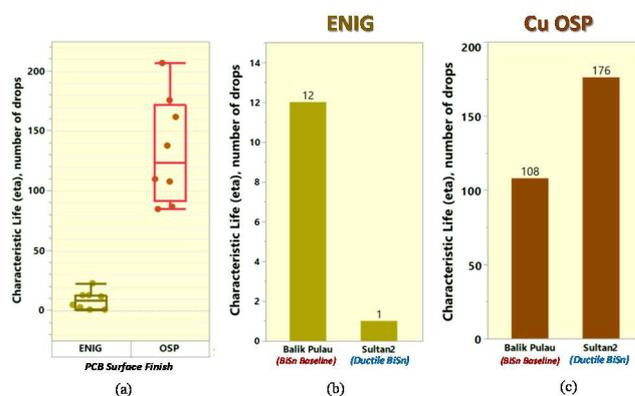
Fig 1. Characteristic Life comparison for FCBGA Solder Joints on Cu OSP and ENIG Surface finishes, between a BiSn baseline solder paste and a ductile BiSn solder paste.
