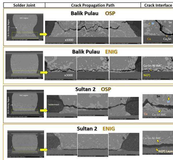
Fig 2. SEM Micrographs depicting the post Mechanical Shock test crack locations for solder joints on the Balik Pulau OSP and ENIG surface finish boards (top two rows) and on the Sultan 2 OSP and ENIG surface finish boards (bottom two rows).
