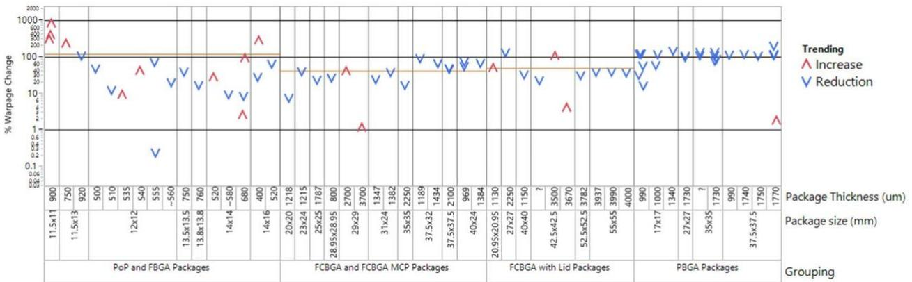
Figure 6. Overall peak reflow warpage reduction percentage
