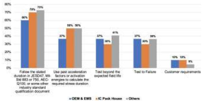
Fig. 6. Practices to Determine the Duration of Stress Test
