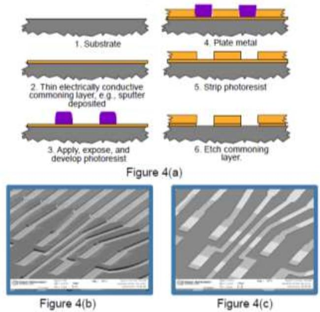
Fig. 4. Semi-Additive Plating Process for Glass TV
