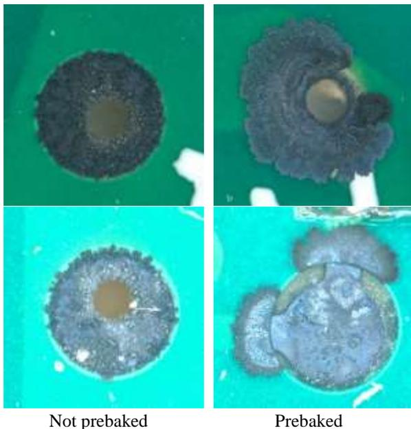
**Figure 7:** Effect of prebaking. Creep corrosion in the FoS test occurred only on PCBs that had been prebaked in flowing N<sub>2</sub> gas at 100°C for 24 hours. [9]
