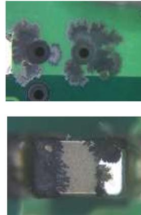
**Figure 8:** 5-day FoS run using KCl saturated solution. The PCB board was prebaked in flowing nitrogen gas at 100°C for 10 hours. The top figure shows creep corrosion on the PCB. The lower figure shows silver migration out of a capacitor termination. The surface mount resistors on the board did not suffer corrosion.
