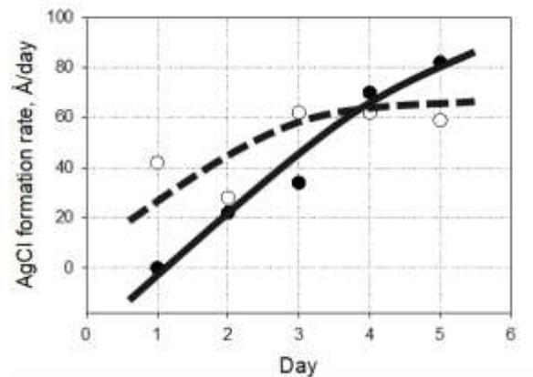
**Figure 4:** The formation rates of AgCl and Ag<sub>2</sub>S are shown as a function of days for Clorox containing 4.12 and 8.25% sodium hypochlorite by the dotted and the solid curve, respectively. The sulfur content was 200 g. The relative humidity was controlled to 59% using sodium nitrite saturated salt solution.
