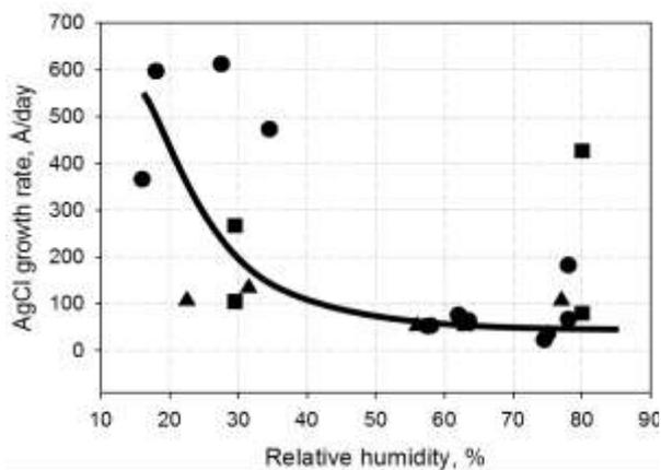
**Figure 5:** Effect of relative humidity on Cu and Ag corrosion rates and AgCl formation rate averaged over a 5-day period. The test was run with 200 g sulfur, 100 ml Clorox™, NaNO<sub>2</sub> saturated salt solution at 50°C. [4]
