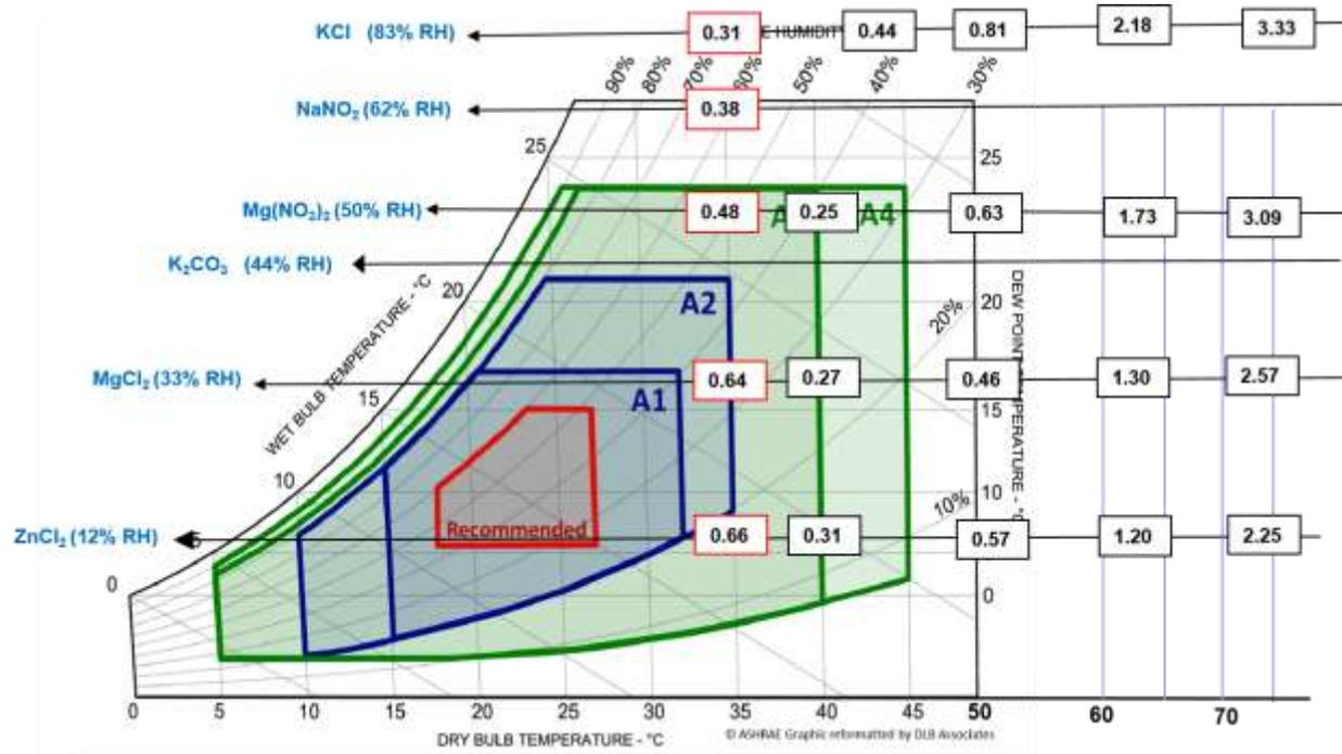
**Figure 9:** The corrosion of serpentine silver thin film can be used to map out the silver corrosion rates across a region of the psychrometric chart of interest. The top right figure shows silver corrosion rate as a function of temperature and relative humidity. The bottom figure shows silver corrosion rates on the psychrometric chart.
