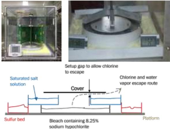
**Figure 1:** iNEMI FoS test chamber loaded with test PCBs. The tray-like setup below the test PCBs provides the sulfur and chlorine gases and maintains the relative humidity in the chamber at the deliquescence relative humidity of the saturated salt solution in the setup. [4]
