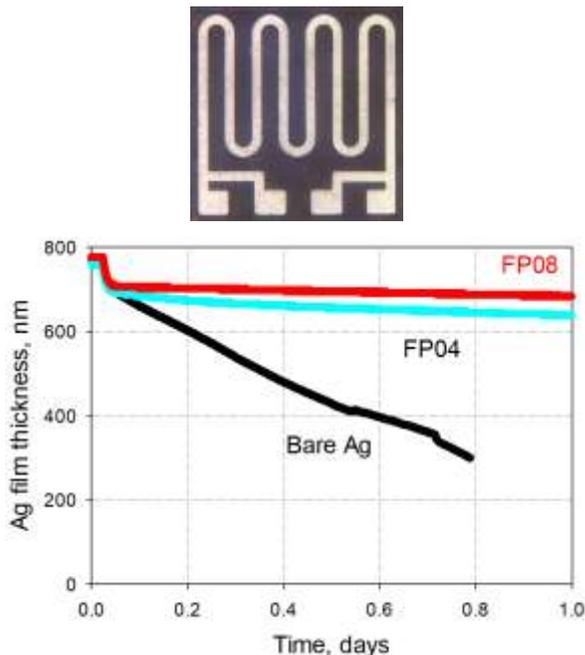
**Figure 10:** Conformal coating characterization can be done by coating a serpentine silver film with the conformal coating of interest and measuring and comparing the corrosion rate of the coated silver to a bare silver thin film. The slope of the curves above are the corrosion rates for thin films coated with FP08 and FP04 conformal coating and a bare thin film. [13] ability of the in the iNEMI FoS chamber to be an industry-
