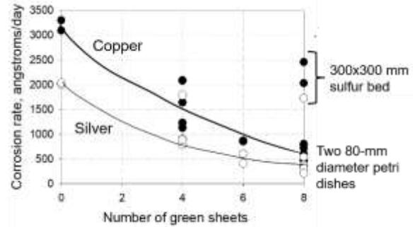
**Figure 6:** The effect of loading (number of PCBs) on copper and silver corrosion rates. The solid dots are for copper corrosion; the open dots for silver corrosion. The green sheets are PCBs. The test was conducted at 50°C chamber temperature. The sulfur was contained in two 80-mm diameter beakers and KCl saturated salt in two 100-ml beakers. No Clorox was used in this test. [10]
