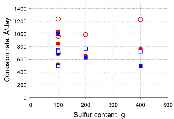
**Figure 2:** Effect of sulfur content on the copper and silver corrosion rates. The red circular dots are for copper corrosion rates and the blue square dots are for silver corrosion rates. The open dots are for mass gain method and the solid dots for coulometric reduction method. The relative humidity of 46-57%, during the test, was maintained using ammonium nitrate saturated salt solution. [3]
